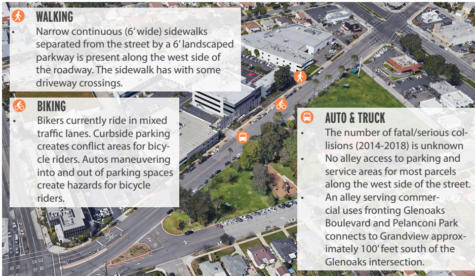
FIG 3.25 EXISTING PROJECT AREA 1 GLENOAKS BOULEVARD TO SAN FERNANDO ROAD – LOOKING NORTH
